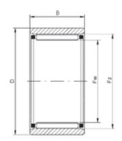
40 mm x 55 mm x 20 mm ISO RNAO40x55x20 cylindrical roller bearings
